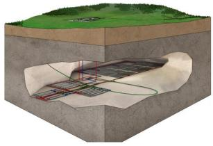
[Addition A shows the design of geologic repository of spent nuclear fuel and HLW]
